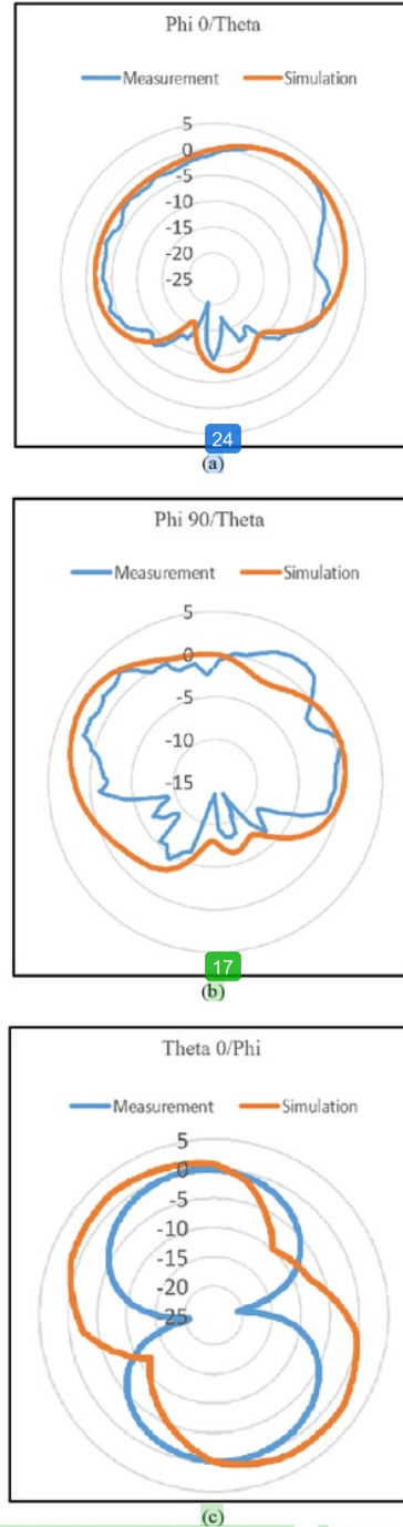
Fig. 9. Simulated & Measured Radiation Pattern at 4.8GHz Frequency (a) XZ plane (b) YZ plane (c) XY plane
